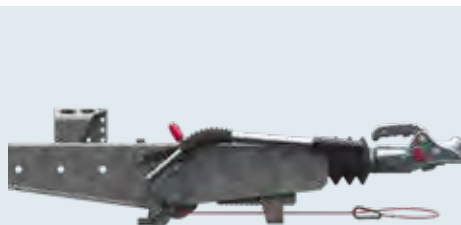
Handbrake lever opened = brake rod not clamped
