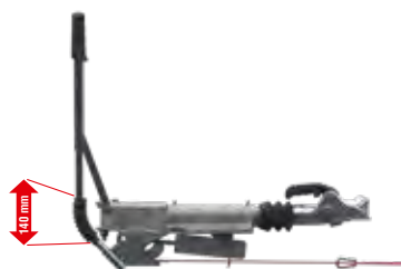
Handbrake lever closed (parking brake backwards, brake optimally set)
