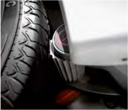
Strong, sturdy, compact: Powerful electric motors in each unit drive the trailer wheels.
