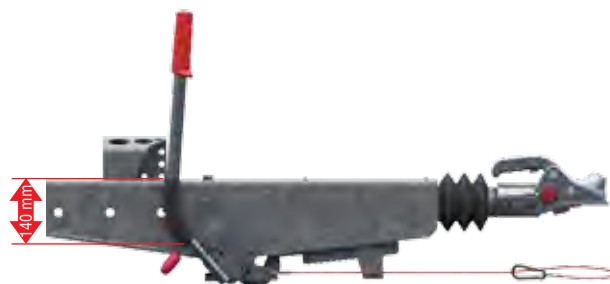
Handbrake lever closed (position with trailer on incline)
