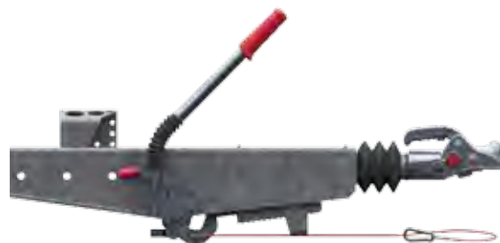
Handbrake lever closed (position with trailer on down-slope)
