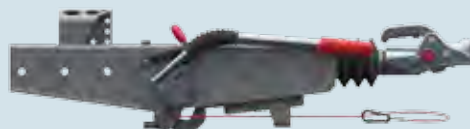
Handbrake lever applied = brake linkage clamped, handbrake lever lowered
