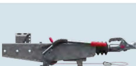
Handbrake lever opened = brake linkage not clamped
