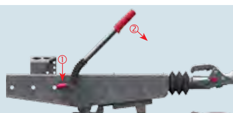
Handbrake lever applied = brake linkage clamped Press the locking lever ① and lower the handbrake lever ② at the same time
